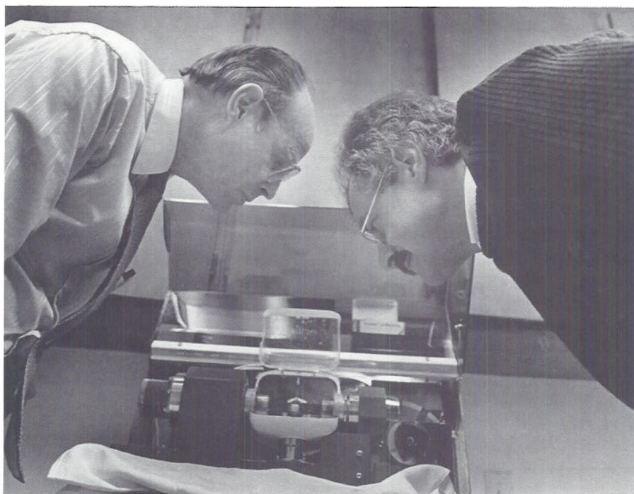
Drs. Preston and Duret watch the CAD/CAM's computer-assisted micro-milling machine in action. The machine uses a series of specialized cutting tools to form a complete restoration from a block of dental material.
