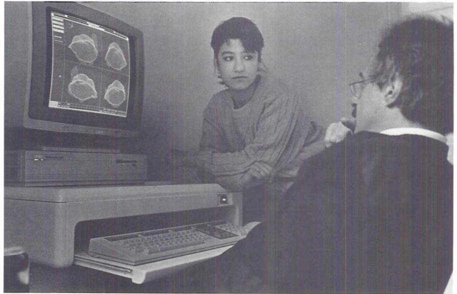
Francois Duret, D.C.D., Ph.D., and research technician Koatherine Pitiot, look over three-dimensional wire-mesh projections of an imaged tooth. The CAD/CAM system developed by Dr. Duret enables the dentist to design and produce a complete restoration entirely by computer.
