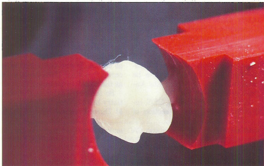
Milling molars: This upper first molar appears at the end of the milling process. It is now ready for removal from the material block. In this case, the crown is made from a new material called Aristee.
