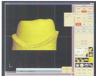
Five axis measurement- model rotation ( \theta ) and 180 degree rotation of the laser sensor ( \alpha ) as well as length, width and height (x, y, z)
