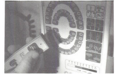
FIG. 13. The generator wired to a remote control.
