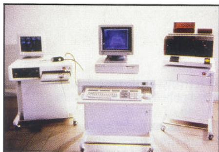
Figure 1. The three units of the CAD/CAM system: from left to right, the image acquisition station, the CAD system, the CAM unit
