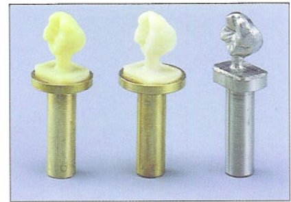
Fig 26 Crowns which have been processed using three kinds of processing materials (left: composite block; middle: ceramic block; right: titanium block).
