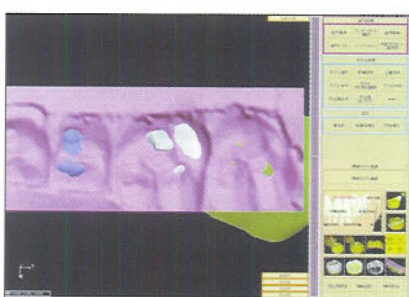
Fig 16 Determination and confirmation of the position and range of the contact point between crown model and the antagonist tooth.
