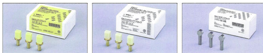
Fig 3 Materials for processing: composite, ceramic, and titanium blocks.
