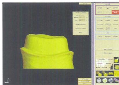
Fig 17 Setting the space for cement.
