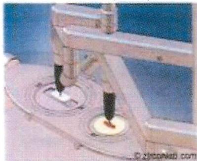
2-3 The ZIRKON ZAHN pantograph by E. Steger.
