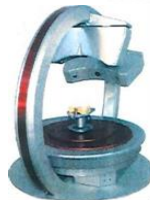
2. In labs equipped with a CAD / CAM system, scanners (here, the Cynoprod i3 Evolution, double head scanner) are extensively used to perform the optical impression on a model transmitted by the surgeon-dentist.
