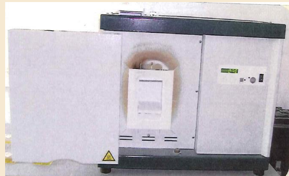
Image 9: Sintering furnace or LAVA® Therm.
