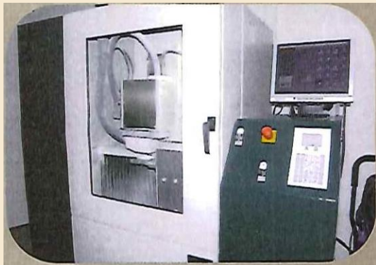
Image 8: The machine-tool or LAVA® Form Milling Unit.
