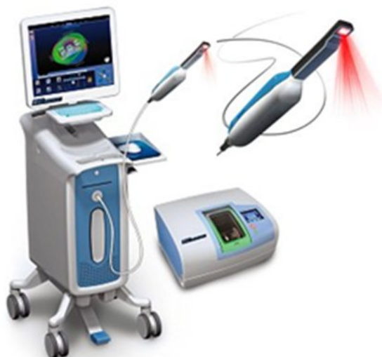
Figure 11- E4D Dentist system, wand and milling unit (27)
